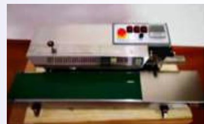
FRD-770 BAND SEALER WITH NITROGEN FLUSH SS HORIZONTAL
