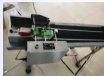
SD-4 STRACKER CONVEYOR WITH TIJ PRINTER
