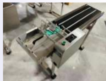
SD-5 STRACKER CONVEYOR WITH TIJ PRINTER
