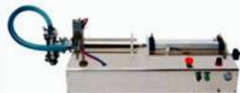
G1WY100 LIQUID FILLING MACHINE 10ML-100ML SINGLEHEAD
